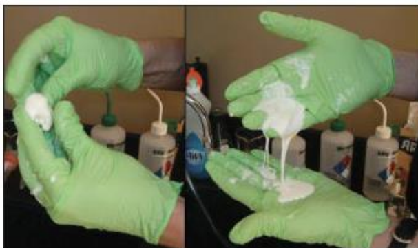
Fig. 1. A cornstarch-water mixture can be rolled around in your hand like a ball of soft clay (left), but will then flow like a liquid when you cease rolling it (right)
